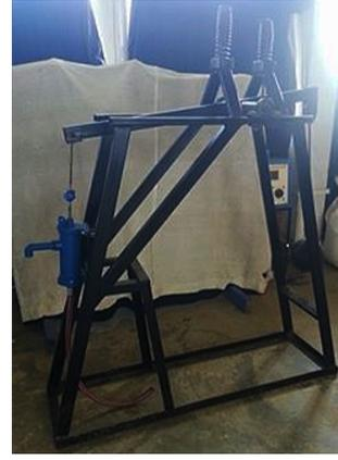
Figure 2: Fabricated pendulum assisted hand water pump.
