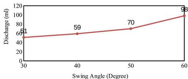
**Figure 3:** Discharge of water from pendulum pump vs. swing angle of pendulum.**Table 3:** Observation of discharge of water from Pendulum pump and Normal water pump.
