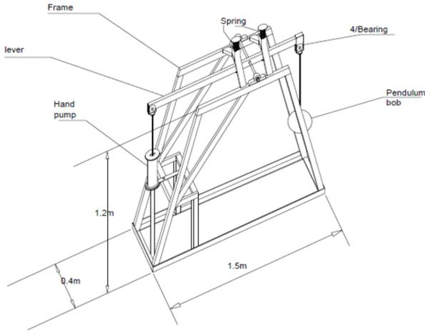
Figure 1: Model of pendulum pump.
